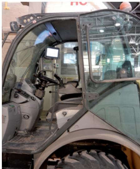
Fig. 3 De shovel with the operators-terminal
