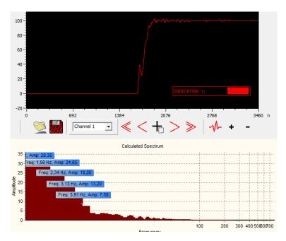
As you can see the graph does not look good, in the spectrum analyzer we can see that a lot of frequencies interfere with the weight signal. We can filter these frequencies out with the cutoff filter.
