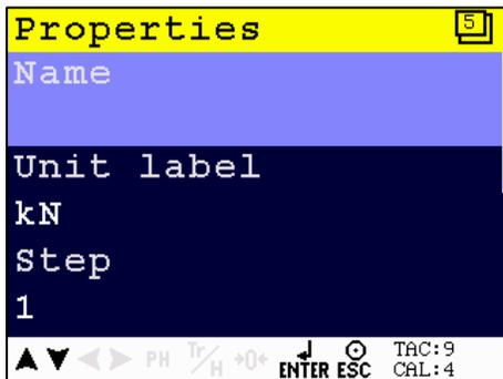
Here the Unit, Step size, Decimal point and Max load can be set
